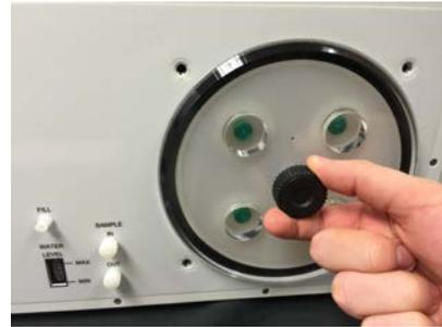
A close-up photograph of a hand unscrewing a black cap from a circular chamber door. The door is white with a black ring around the opening. To the left of the door, there are two white knobs labeled 'FULL' and 'SAMPLE', and a small black switch. | <p><b>Open the Chamber Door</b></p> <p>Unscrew any visible fasteners and pull the door from the chamber with moderate force.</p> |
