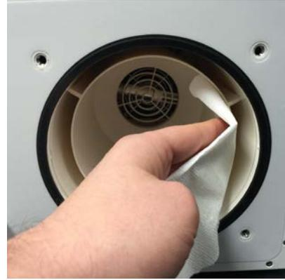
A close-up photograph of a hand using a white paper towel to clean the interior of the chamber door. The door is white with a black ring around the opening. The interior of the door is visible, showing a circular fan or vent.                     | <p><b>Clean With Paper Towel</b></p>                                                                                             |
